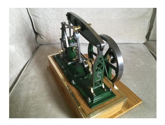
Working from scaled plans Stephen machined the components from stock metal to complete the model
